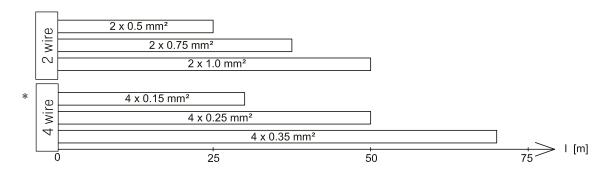
Please note that flow and return sensors must be connected with equally long cables when using two-wire connection.
