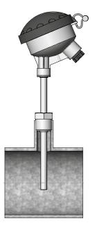
**Example 2**Pocket sensor mounted in "T" with 45° angle.
